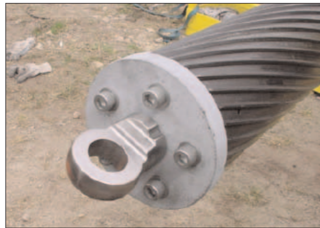
Left : Eyebolt in the tipcontrol of a 1,5 MW turbine, first design. The eyebolt detached, caused two heavy damages of blades and had to be replaced in the whole series - "retrofitting". On the right the "new" eyebolt.
